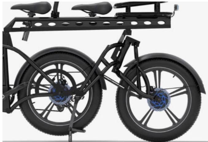
The right brake lever controls the middle and rear brake
