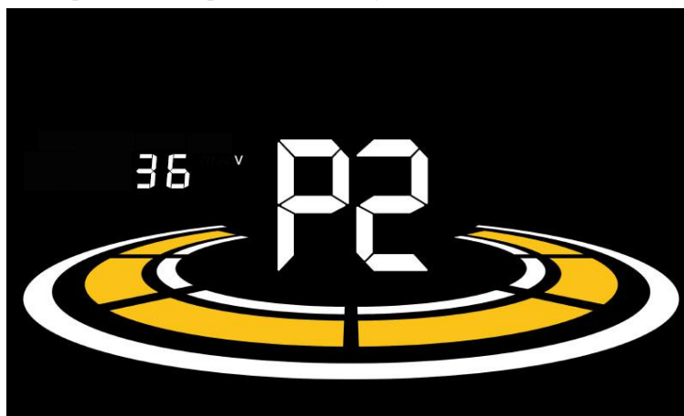
Figure 6-2 Rated voltage setting interface
